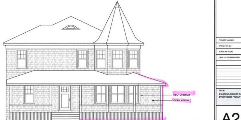
EXISTING FRONT ELEVATION PROPOSED FRONT ELEVATION
