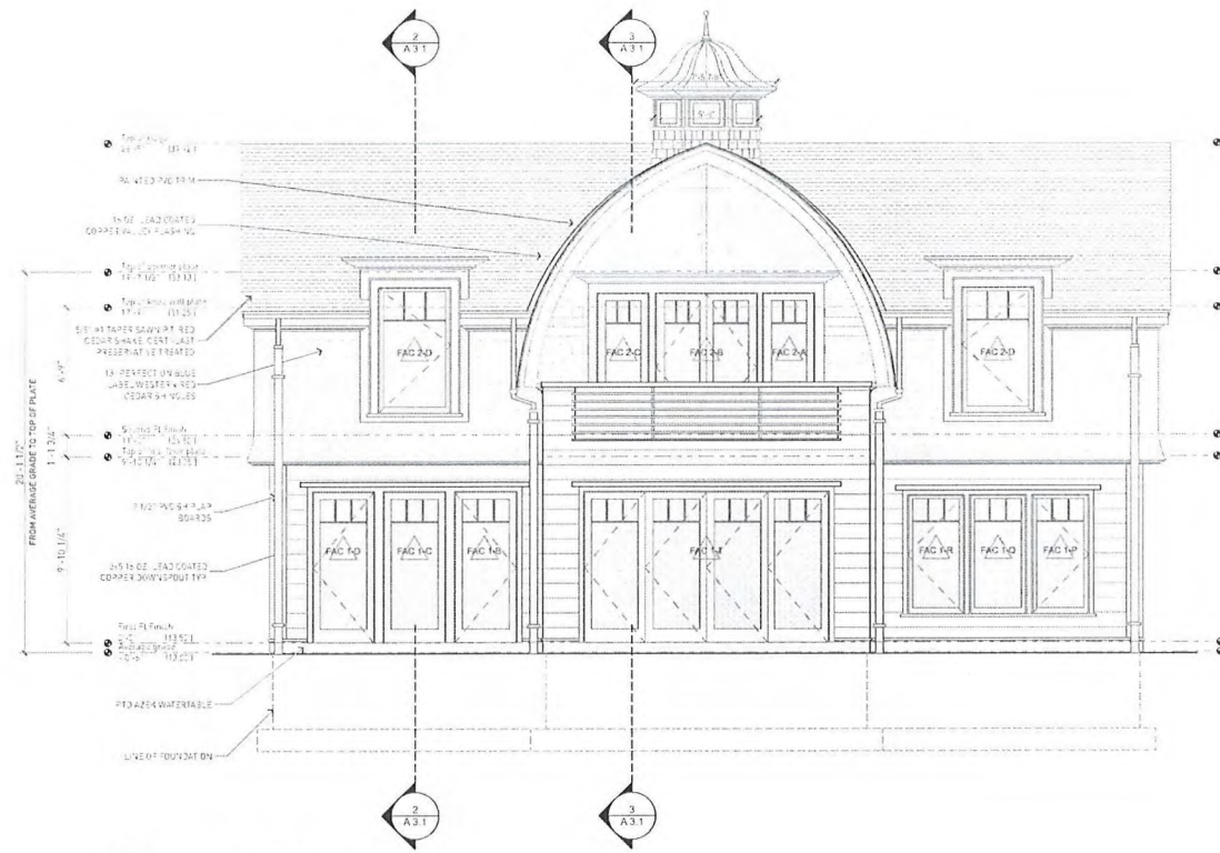
1 South Elevation SCALE: 1/4" = 1'-0"
